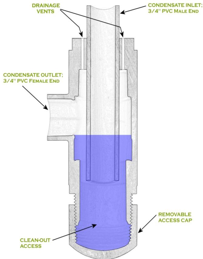
The top inlet is a  $\frac{3}{4}$ " male end, intended to be connected (*using PVC glue*) to any  $\frac{3}{4}$ " PVC female fitting (*i.e. coupling, 45° or 90°, male or female adaptors, etc.*) at the outlet of a condensate drain pan of any equipment that produces and accumulates condensation (*such as an evaporator coil*).
